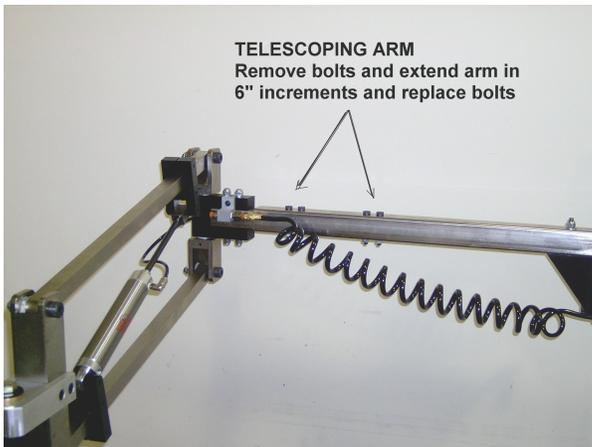
TELESCOPING 12 GA STEEL TUBING PERMITS EASY LENGTH ADJUSTMENT WHILE MAINTAINING STRENGTH INTEGRITY
